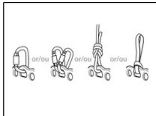
The hole design allows ropes or slings to be threaded for direct connection.
